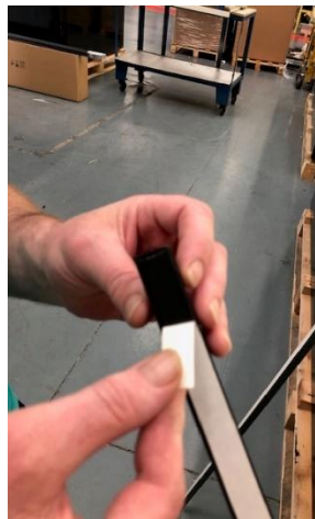
Remove backing from double sided sponge tape
